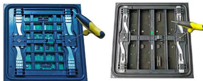
Rear side PCB With coating
